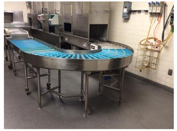
New cove base. Grout lines completely eliminated. Better COF (Slip Coefficient).
