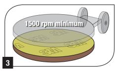
Burnish the floor with 3M<sup>™</sup> Scotch-Brite<sup>™</sup> Sienna Diamond Floor Pad. Use a high speed machine (1500 rpm minimum) for 6 passes.
