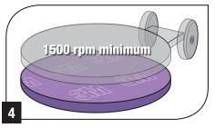
Burnish the floor with dry **3M™ Scotch-Brite™ Purple Diamond Floor Pad**. Use extra high speed machine (1500 rpm minimum) for 6 passes.
