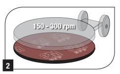
Clean the floor with **3M**<sup>™</sup> **Surface Preparation Pad** using only water. Use low/standard speed machine (150-300rpm). Make 6 passes using plenty of water. To finish, remove water and dry the floor.
