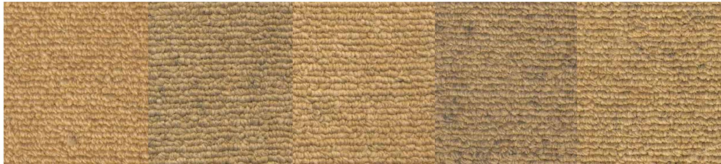
A competitive type 6,6 nylon trilobal with a generic soil resistance treatment
